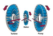
Turbine is directly connected to the engine flywheel, so it spins at the same speed. The stator is the middle part that will redirect the fluid from the turbine to the pump, forcing this one to rotate nearly at the same speed as the turbine that will transmit the movement forward as it's directly connected to the transmission. In low engine rpm's the force of the fluid is so low that almost no rotation will be generated in the pump.
