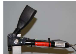
Figure 10 – Buckle after pretensioner activation [4]
