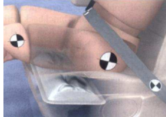
Figure 33 – Seat with airbag “anti-submarine” effect [10]
