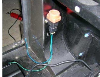
Figure 34 – Fuel cut-off reset switch [16]
