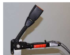
Figure 9 – Buckle before pretensioner activation [4]
