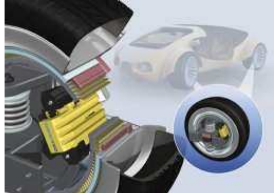
Figura 2: Motor in-wheel mounted
