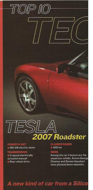
It has lithium-ion batteries and comes with a charging cable, just lik your cellphone. Unlike your phone, however, it can go from zero t IOO kilometers per hour in less than 4 seconds, pinning you agains the back of your seat like a fighter pilot. And it'll do it with a lot les noise—and for US \$70 000 less—than a Ferrari F430.
