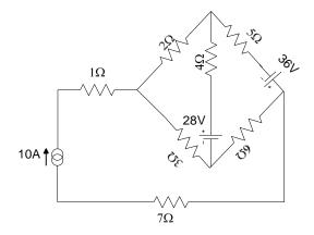
$(Sol:\ I_1=10A,\ \ I_2=4.42A,\ \ I_3=5.58A,\ \ I_4=-5.02A,\ \ I_5=9.44A\ ,\ \ I_6=0.56A)$
