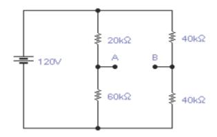
$$V_{Th} = V_{AB} = V_{40k} - V_{20k}$$
