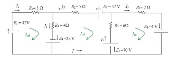
$$\begin{cases} E_1 + E_4 = (R_1 + R_4) \cdot I_{m_1} - R_4 \cdot I_{m_2} \\ -E_4 - E_2 - E_5 = -R_4 \cdot I_{m_1} + (R_4 + R_2 + R_5) \cdot I_{m_2} - R_5 \cdot I_{m_3} \\ E_5 + E_3 = -R_5 \cdot I_{m_2} + (R_5 + R_3) \cdot I_{m_3} \end{cases}$$
