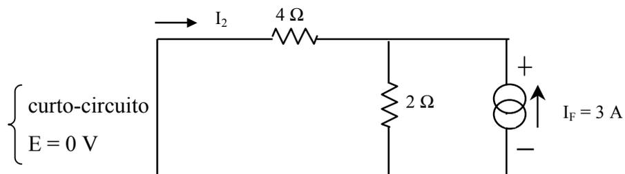
$$\text{Divisor de corrente} \quad \rightarrow \quad I_2 = - I_F \frac{2}{4 + 2} = -1 \text{ A}$$
