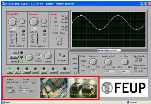
Figure 10. Experiment interface window #2 for parametric testing: Oscilloscope, waveform generator, multimeter, live images from the remote lab. Notice that the oscilloscope and the waveform generator are not used in this experiment.
