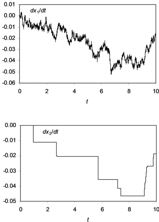
**Fig. 2 Time history of  $\dot{x}_1$  and  $\dot{x}_2$  for one simulation with  $T_w=10.0$  s,  $F_{\max}=10.0$  N,  $M_1=M_2=1.0$  kg,  $h=10^{-2}$  m,  $dt=5.0 \times 10^{-6}$  s**
