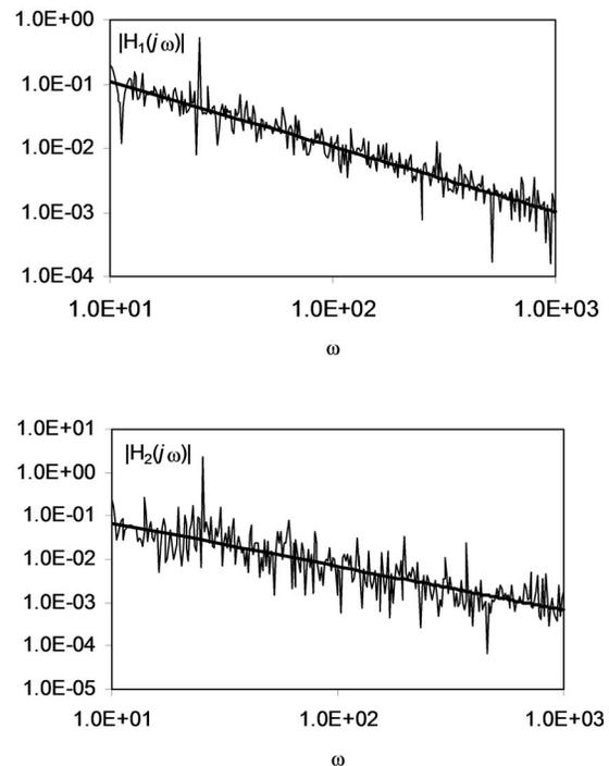
**Fig. 3 Transfer functions  $H_1(j\omega)$ ,  $H_2(j\omega)$  and approximations  $\{m_1^{-1}, \alpha_1\} \approx \{1.18, -1.02\}$  and  $\{m_2^{-1}, \alpha_2\} \approx \{0.71, -1.01\}$ , for one simulation with  $T_w=10.0$  s,  $F_{\max}=10.0$  N,  $M_1=M_2=1.0$  kg,  $h=10^{-2}$  m,  $dt=5.0 \times 10^{-6}$  s**
