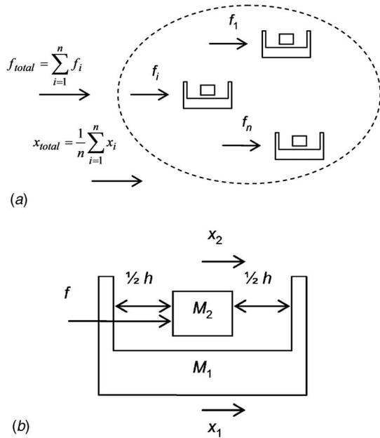
**Fig. 1 Mechanical system; (a) multicomponent global structure and (b) elemental component, with two masses  $M_1$  and  $M_2$  with backlash  $h$ , subjected to impacts under the action of force  $f$**
